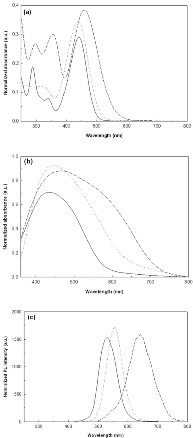
**Fig. 3.** Absorption spectra of **R1** (—), **R2** (...), and **R3** (---) (a) in  $\text{CH}_3\text{CN}$  and (b) absorption on  $\text{TiO}_2$  film. (c) Emission spectra of **R1** (—), **R2** (...), and **R3** (---).
