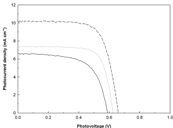
**Fig. 8.** Current density-voltage characteristics for **R1** (—), **R2** (...), and **R3** (---) DSSCs under illumination of simulated solar light (AM 1.5, 100 mW cm<sup>-2</sup>).
