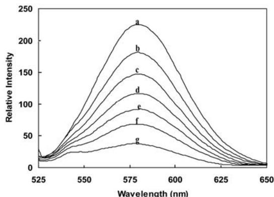
**Fig. 7.** Emission spectra of EB (5  $\mu\text{M}$ ) bound to DNA (12  $\mu\text{M}$ ) in 7.5 mM phosphate buffer (pH 7.2) at  $\lambda_{\text{ex}}=510$  nm in the absence (a) and presence of varying concentrations of TMPyP: 0.15  $\mu\text{M}$  (b), 0.3  $\mu\text{M}$  (c), 0.45  $\mu\text{M}$  (d), 0.60  $\mu\text{M}$  (e), 0.75  $\mu\text{M}$  (f) and 0.90  $\mu\text{M}$  (g).
