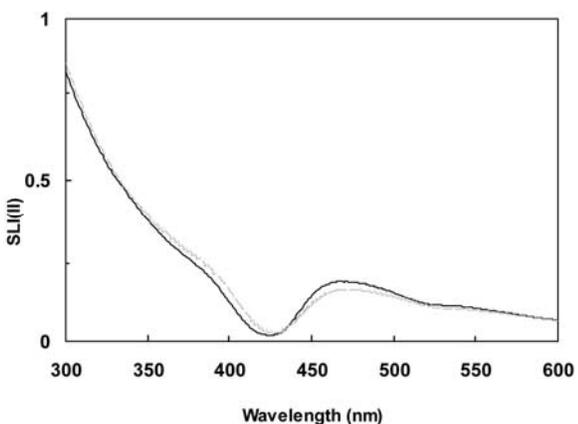
**Fig. 11.** Light scattering profiles of 5.3  $\mu\text{M}$  of 5-CBPpP in 7.5 mM phosphate buffer (pH 7.2) in the absence (—) and presence of 2 M of NaCl (----).
