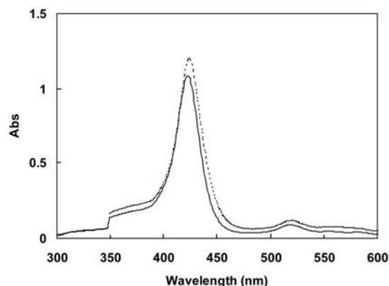
**Fig. 1.** UV-Vis spectra of TMPyP at constant concentration of 3  $\mu\text{M}$  in 7.5 mM phosphate buffer (pH 7.2) in the absence (—) and presence of 2 M NaCl (----).
