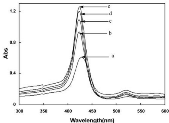
**Fig. 5.** UV-Vis spectra of DNA/TMPyP solution (at a molar ratio of 2.28) 5.3  $\mu\text{M}$  5-CBPpP in 7.5 mM phosphate buffer (pH 7.2) in the absence (a) and presence of varying concentrations of NaCl: 0.28  $\mu\text{M}$  (b), 0.75  $\mu\text{M}$  (c), 1.12  $\mu\text{M}$  (d) and 1.98  $\mu\text{M}$  (e).
