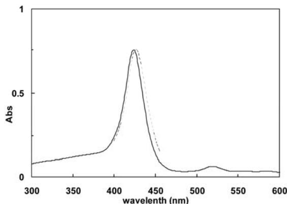
**Fig. 2.** UV-Vis spectra of 5-CBPyP at constant concentration of 5.3  $\mu\text{M}$  in 7.5 mM phosphate buffer (pH 7.2) in the absence (—) and presence of 2 M NaCl (----).
