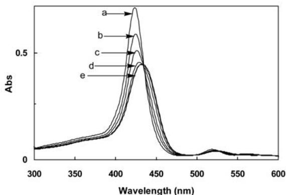
**Fig. 4.** UV-Vis spectra of 5.3  $\mu\text{M}$  5-CBPyP in 7.5 mM phosphate buffer (pH 7.2) in the absence (a) and presence of varying concentrations of calf thymus-DNA: 1.98  $\mu\text{M}$  (b), 13.9  $\mu\text{M}$  (c), 15.9  $\mu\text{M}$  (d), 17.9  $\mu\text{M}$  (e).
