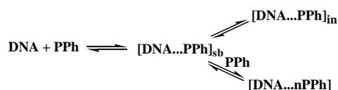
where  $[\text{DNA}\dots\text{PPh}]_{\text{sb}}$ ,  $[\text{DNA}\dots\text{PPh}]_{\text{in}}$  and  $[\text{DNA}\dots\text{nPPh}]$  represent the superficially bound, the intercalation binding, and aggregation (self stacking) porphyrin molecules, respectively.
