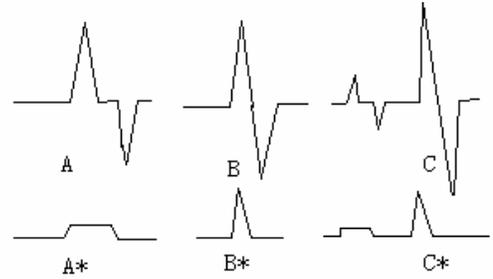
**Fig. 1.** Conventional and derivative signal of FAAS: (A\*) FAAS, (B\*) FI-FAAS, (C\*) AT-FAAS, (A) D-FAAS, (B) D-FI-FAAS, (C) D-AT-FAAS.
