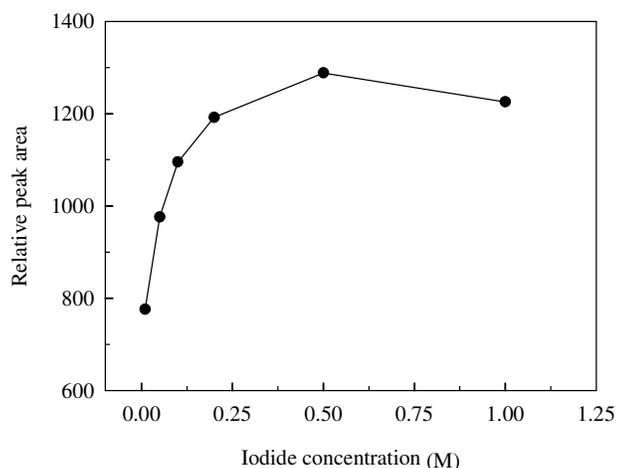
**Fig. 3.** Effect of iodide concentration on the chemiluminescence signal.  $\text{H}_2\text{SO}_4$ , 0.5 M;  $\text{NO}_2^-$ ,  $1 \mu\text{g ml}^{-1}$ .
