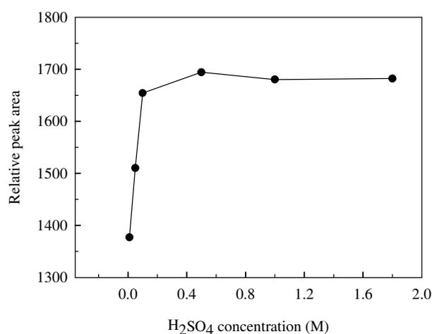
**Fig. 2.** Effect of sulfuric acid concentration on the chemiluminescence intensity.  $\text{NO}_2^-$ ,  $1 \mu\text{g ml}^{-1}$ .
