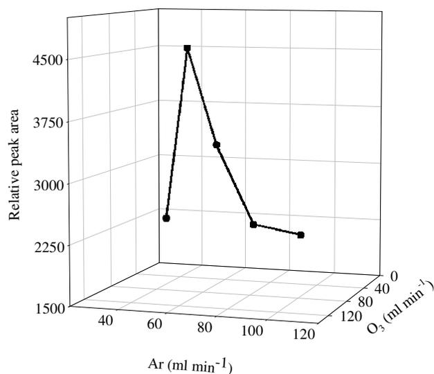
**Fig. 4.** The influence of argon and ozone flow rates on the chemiluminescence response.  $\text{H}_2\text{SO}_4$ , 0.5 M;  $\text{NO}_2^-$ ,  $1 \mu\text{g ml}^{-1}$ .
