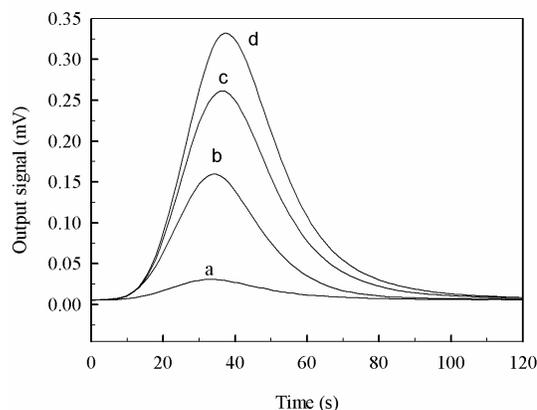
**Fig. 6.** Typical smoothed curve of chemiluminescence signals recorded at (a) 0.10, (b) 0.50, (c) 0.80 and (d) 1.0  $\mu\text{g ml}^{-1} \text{NO}_2^-$  at optimized conditions.
