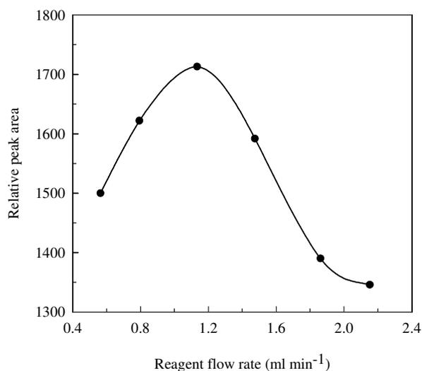
**Fig. 5.** Effect of flow rate of reagents in the flow injection procedure.  $\text{H}_2\text{SO}_4$ , 0.5 M;  $\text{NO}_2^-$ ,  $0.5 \mu\text{g ml}^{-1}$ .
